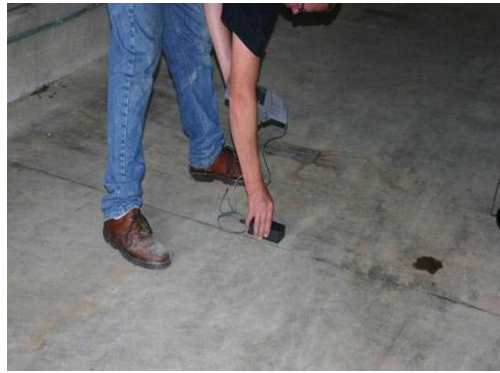
Locating rebar in floor
