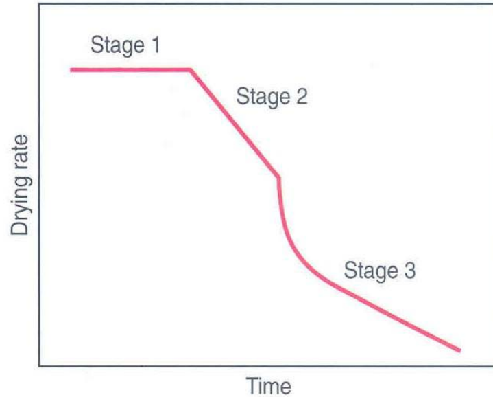
Figure 11. The drying rate trends for the three stages of the drying of concrete. The rate of the first stage depends mostly on temperature, relative humidity, and air flow and is fairly constant. The rates of the second and third stages are more dependent on the cement paste [4].
