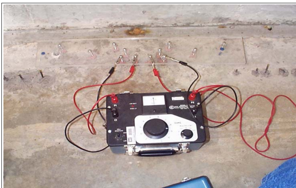
Figure 44. East concrete floor measurement being taken using the Wenner four-pin method.
