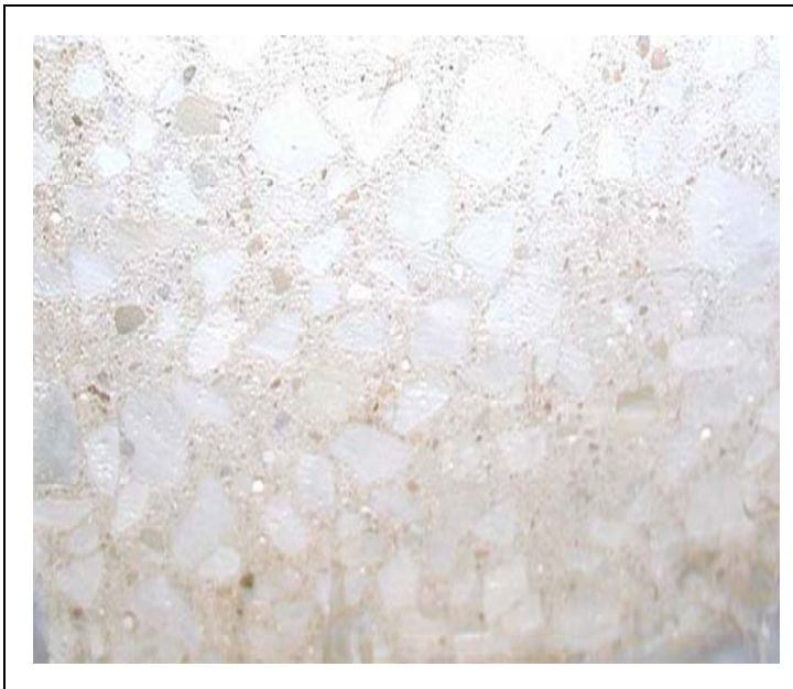
Figure 29. Anode side face before EO experiment for the 5-cm, 0.63 w/c specimen.
