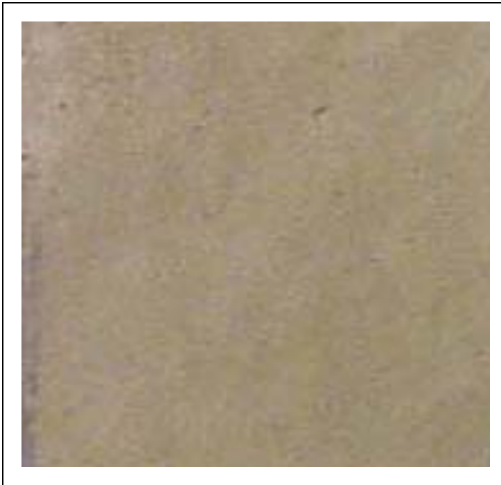
Figure 27. Cathode side face before EO experiment for the 5-cm, 0.63 w/c specimen.
