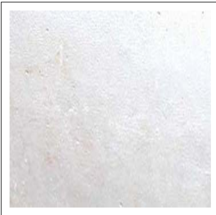
Figure 25. Cathode side face after EO experiment for the 10-cm, 0.63 w/c specimen.
