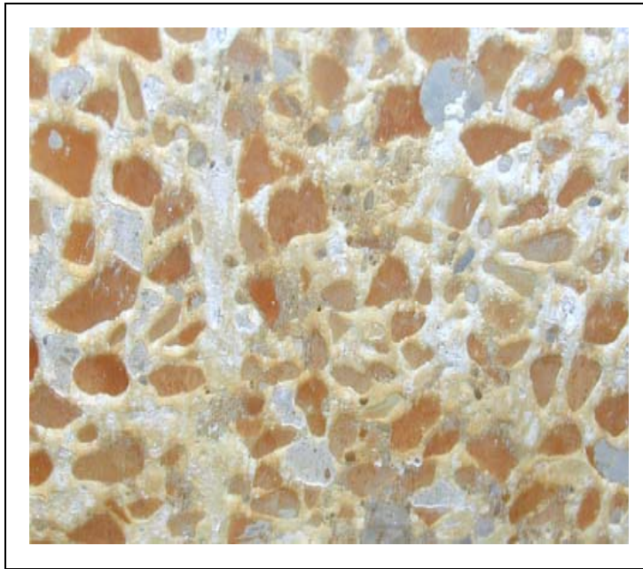
Figure 30. Anode side face after EO experiment for the 5-cm, 0.63 w/c specimen.
