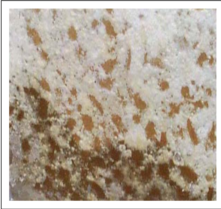
Figure 26. Anode side face after EO experiment for the 10-cm, 0.63 w/c specimen.
