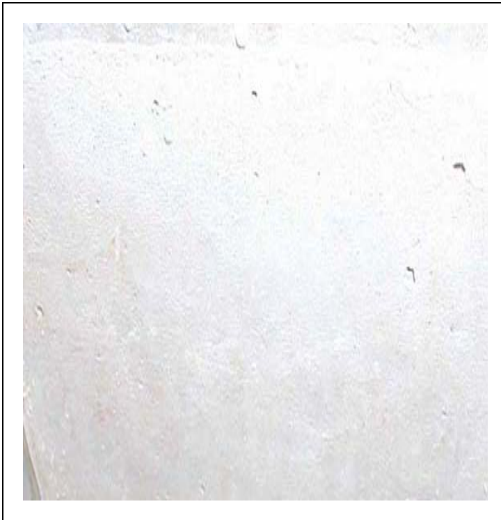
Figure 28. Cathode side face after EO experiment for the 5-cm, 0.63 w/c specimen.
