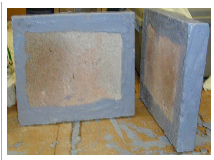
Figure 14. CMU with epoxy sealant before tank placement.
