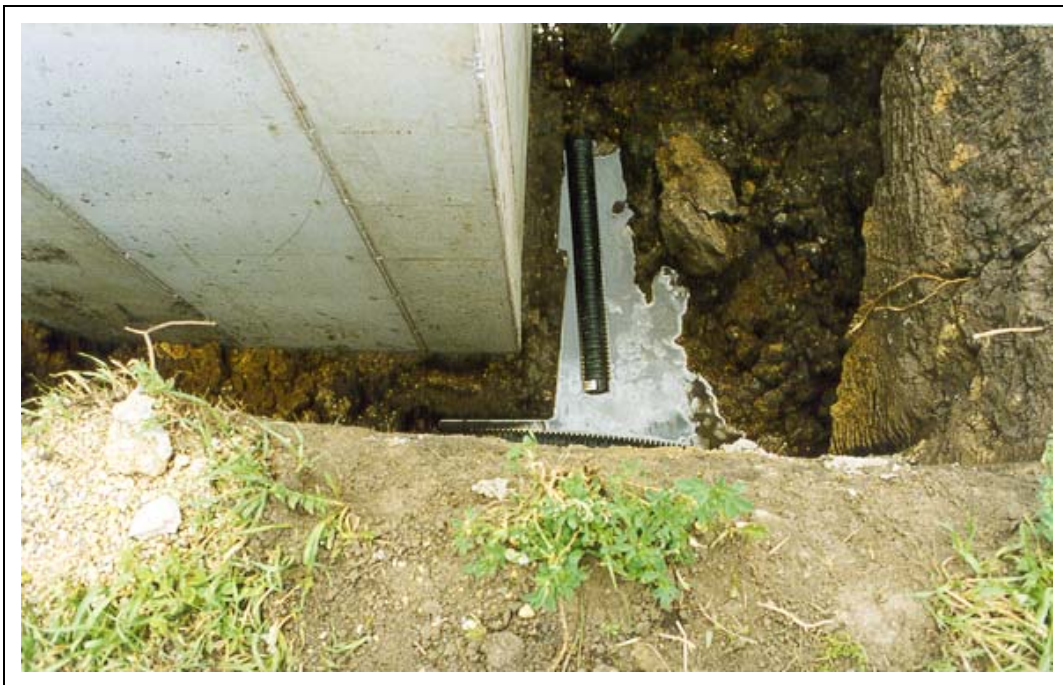
Figure D3. View of the trench surrounding the concrete basement before covering with backfill. The tile at the bottom was used to deliver additional water to raise the water level, allowing some control over the local water level conditions; similar drain tile was installed in the block basement.
